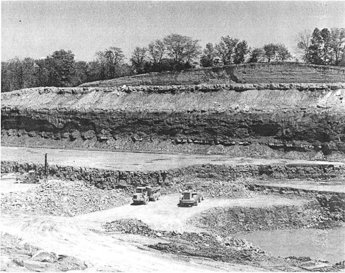
Plate 1. Drilling and loading operations in the upper Plattsmouth limestone at the Ideker Amazonia Quarry. An extensive bench is developed on top of the Kereford limestone behind the track drill. The Kereford face is identified by a red "K" on the right side of the photograph. Photograph courtesy of the Missouri Department of Transportation.
